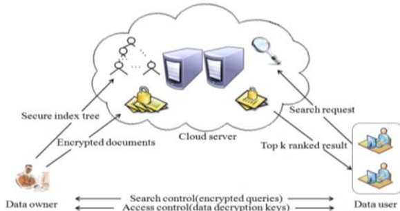
Figure 1: Searchable Encryption Architecture using CRSA
